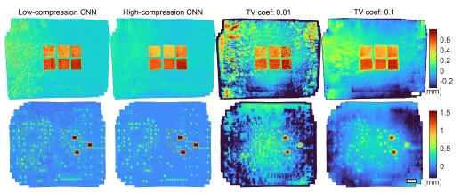
Figure 8. Height map reconstructions of the cut cards and PCB samples using high- and low-compression CNNs (architectures 1 and 4; see supplement for architectures and additional results) and high and low levels of total variation (TV) regularization. Zoom in to see fine features. Scale bars, 1 cm.
