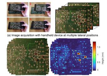
(b) Stitched orthomosaic and height map with 10s of µm accuracy Figure 1. Our method jointly stitches multi-megapixel images acquired under freehand motion at close range and reconstructs high-accuracy height maps without precalibration of camera distortion.
