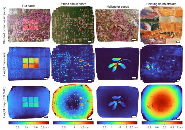
Figure 4. Stitched orthomosaics and height maps for various samples with mm-scale height variation. Height values for the cut cards and PCB components (red ×'s) are quantified in Tables 1 and 2, respectively. COLMAP consistently underestimates heights. Scale bars, 1 cm.
