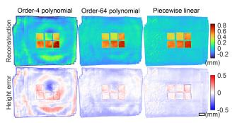
Figure 5. Visual comparison of height map reconstructions of the cut cards sample using different undistortion models. Note the ring artifacts with the polynomial models. Scale bar, 1 cm.
