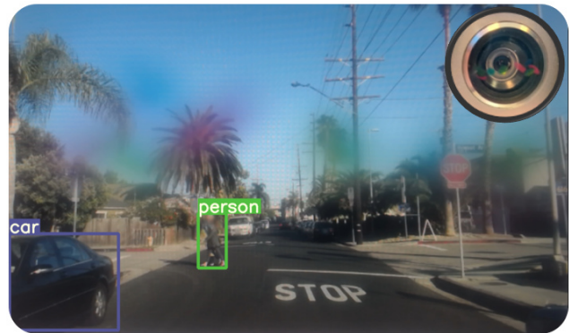
Figure 1: Illustrating the physical translucent patch, placed on the camera lens, which results in the failure to detect the stop sign while correctly identifying the other objects.
