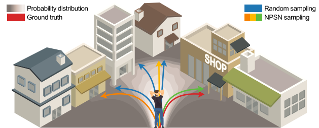
Figure 1. An illustration of a probability distribution of stochastic trajectory prediction and selected paths from each sampling method. While the trajectories from the random sampling are biased in that they do not consider space of all possible distributions, our NPSN purposively generates the accurate route, turning to SHOP, even with its low probability.
