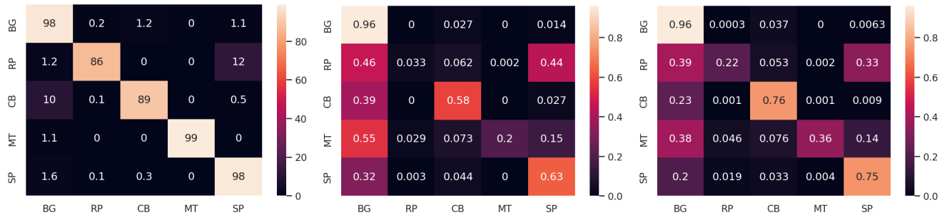
Figure 7. Left: Semantic segmentation confusion matrix of the manual annotations over 20 frames represents human expert agreement after expert review, with the average pixel-level agreement above 94% (see Figure 16 of the Supplementary for the corresponding confusion matrix before expert review). Center: Confusion matrix of DeepLabV3+ on the test split of ZeroWaste-f . Right: Confusion matrix of DeepLabV3+ on the test split of ZeroWaste-f when trained on ZeroWasteAug .
