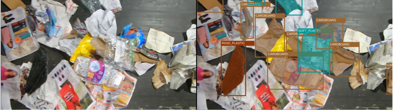
Figure 2. Left: example of an image from ZeroWaste-f dataset. Right: the corresponding ground truth instance segmentation. At the end of this conveyor belt, only paper objects must remain. Therefore, we annotated the removable objects of four material types as foreground: soft plastic, rigid plastic, cardboard and metal. The background includes the conveyor belt and paper objects. Severe clutter and occlusions, high variability of the foreground object shapes and textures, as well as severe deformations of objects usually not present in other segmentation datasets, make this domain very challenging for object detection. More examples of our annotated data can be found in Section 7.3 of the Appendix ( best viewed in color ).
