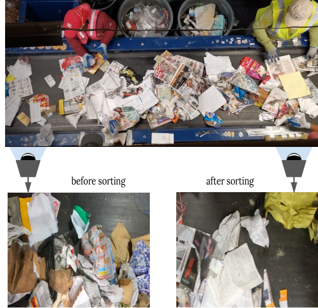
Figure 6. We installed two stationary cameras above the conveyor belt: one at the beginning of the line and another one at the end. At this particular conveyor belt, workers are asked to remove objects of any material other than paper, such as cardboard, plastic and metal. Therefore, the footage collected from the beginning of the line contains the “foreground” objects that need to be removed, and the frames from the end of the conveyor belt are supposed to only contain the “background” paper objects. We used this setup as a foundation of our ZeroWaste- w dataset.
