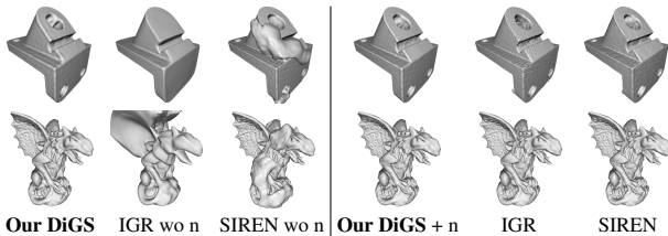
Figure 6. Qualitative results of surface reconstruction on the anchor and gargoyle shapes from the Surface Reconstruction Benchmark [7] compared to state of the art approaches (IGR, SIREN) that use normal vectors as ground truth.
