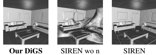
Figure 8. Qualitative results of scene reconstruction. SIREN (right) provides high level of detail, however, when normal vectors are not available (center) the proposed divergence constraint (left) demonstrates a significant improvement.
