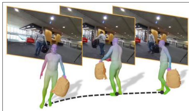
Figure 1. Given a multi-view RGBD sequence, our method tracks the human, the object and their contacts in 3D.
