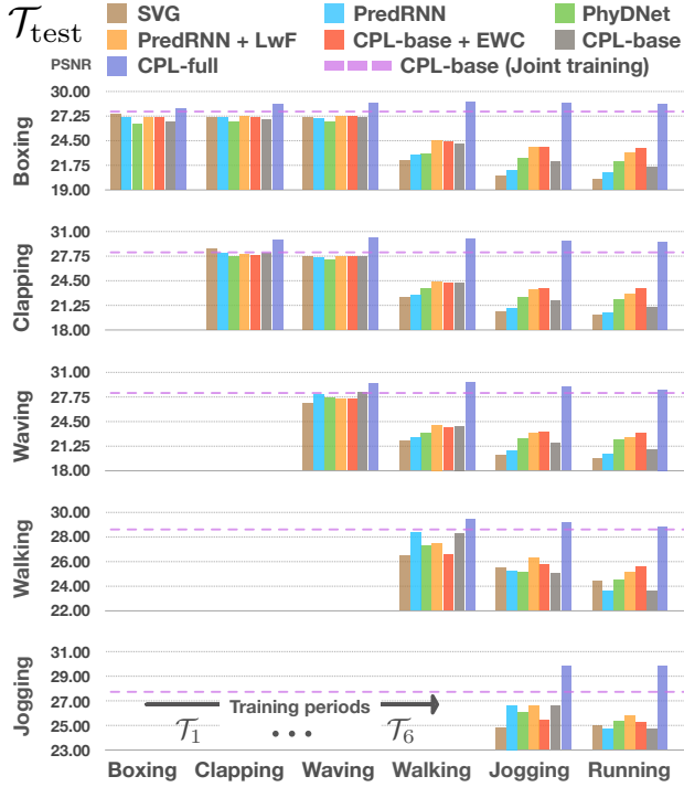
Figure 5. Results on the KTH benchmark. The horizontal axis represents the sequential training process, and the vertical axes represent test results on particular tasks after each training period.
