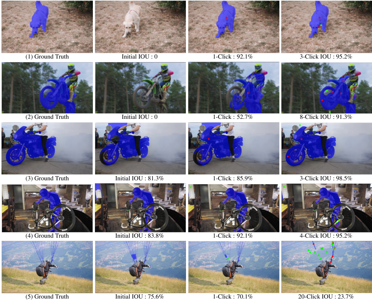
Figure 5. Qualitative results on DAVIS-585 benchmarks. The results are predicted by FocalClick-B3-S2. Row 1, 2 show the example of annotation from scratch. Row 3, 4 demonstrate the cases starting from initial masks. Row 5 shows the bad cases.
