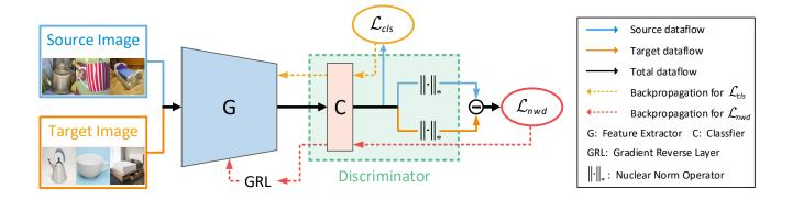
Figure 2. An overview of the adversarial paradigm in the form of DALN, which consists of a feature extractor G and a task-specific classifier C.  $\mathcal{L}_{cls}$  is used to guarantee a low source risk for the source domain, and  $\mathcal{L}_{nwd}$  is used to empirically estimate the NWD that can be coupled with classifier C to implicitly serve as a discriminator. The gradient reverse layer is used to help perform the adversarial learning.
