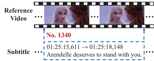
Figure 2. An example of how to cut a movie into a series of video clips according to SRT subtitle files. Note that the SRT files contain both starting and ending time-stamps for each video clip. No. 1340 refers to the sequential number of the current utterance.
