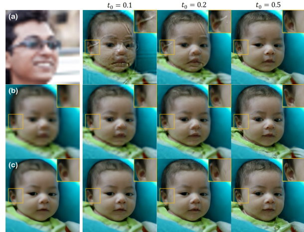
Figure 3. Stability of convergence depending on the choice of initialization. (a) Random initialization, large \varepsilon_0 , (b) vanilla initialization, moderate \varepsilon_0 , (c) NN initialization, small \varepsilon_0 .
