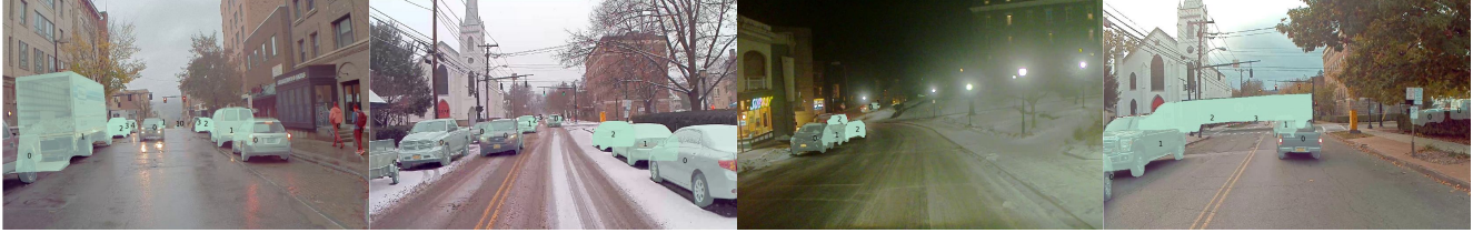
Figure 5. Examples of amodal ground truth masks for cars across different weather conditions.
