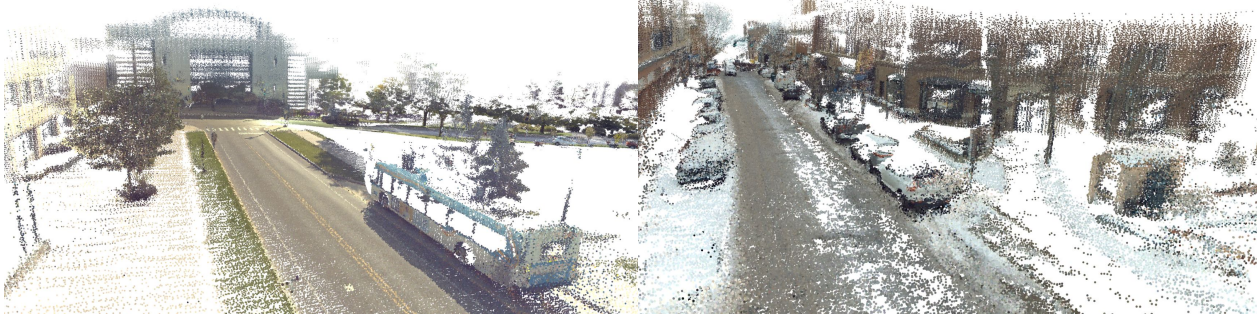
Figure 1. Point clouds generated using calibrated images, LiDAR points, and GPS/IMU data. Left: Point cloud from a sunny day while driving near buildings on campus. Right: Point cloud from a snow day (i.e., white on the road) through an urban portion of the route.
