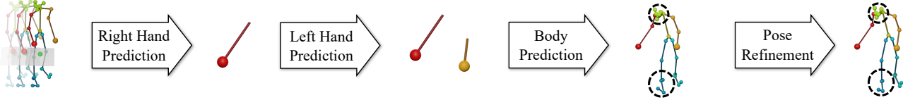
Figure 4. To model joint dependencies within the human skeleton, we sample joints in an autoregressive manner by first predicting the end-effectors (right and left hand), then the rest of the body; pose refinement then improves skeleton consistency.
