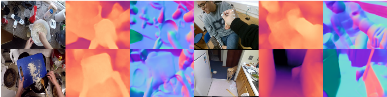
Figure 1. We study the problem of predicting geometry (depths and surface normals) from a single view egocentric image that includes dynamic objects (e.g., hand and people). We design a multimodal spatial rectifier that can effectively handle the excessively tilted images caused by head movement (e.g., nearly 90 degree pitch angle when engaging eye-hand coordination). Our method shows strong performance on unseen images from EPIC-KITCHENS [7] (left), FPHA [18] (top right), and our EDINA (bottom right) datasets.
