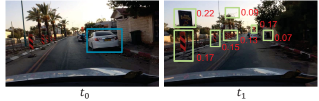
Figure 3. The dissimilarity measurement. For each ID object at timestamp t_0 (in blue), we discover the objects in the reference frame that are dissimilar to it (in green), which are more likely to contain OOD objects for model regularization. The red numbers show the dissimilarity after normalization (Equation (2)).
