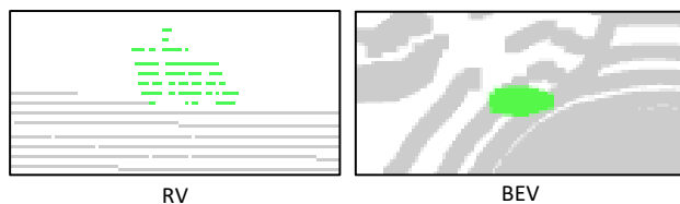
Figure 9. Comparison of point cloud representation in BEV and RV planes for a motorcycle. Best viewed in color.
