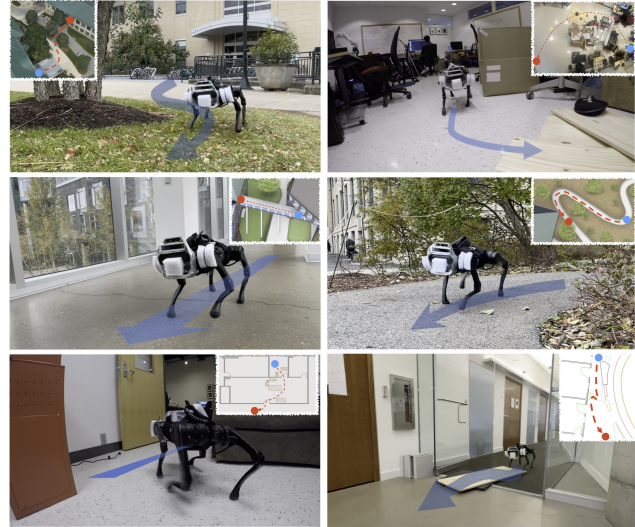
Figure 1. Example deployment scenarios for our proposed point goal navigation system for legged robots. The varying terrains on the way to the goal require the planner to be aware of the robot’s locomotion capabilities. The proprioceptive coupling between the locomotion controller and the navigation planner allow the robot to sense properties of the environment which the vision might miss (slippery terrain, glass obstacle, etc.).
