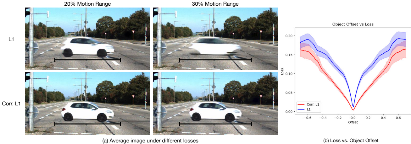
Figure 2. The effect of positional errors on different losses. (a) We show images that minimize the expected error for a toy video prediction task. The car’s location is sampled uniformly about the center at random (either 20% or 30% of the image width). The full range of the car’s locations is indicated by the black bars. Note that the L_1 loss predictions are blurry, in particular for the 30% setting, whereas the correspondence-wise L_1 loss predictions are crisp in both cases. (b) We examine how the loss changes as a function of positional error (i.e., how far the predicted object is from its true location). Correspondence-wise losses increase smoothly with magnitude of the error.
