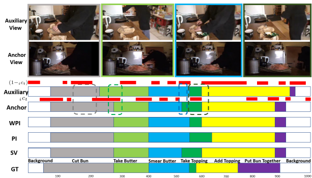
Figure 7. Pseudo ground-truth generated by 3 multi-view inference techniques during training. The red bar above each single-view inference result (anchor/auxiliary) indicates their learned view confidence weight c_t at each frame. Each pair of frames corresponds to the time enclosed by its color-coded dashed box.
