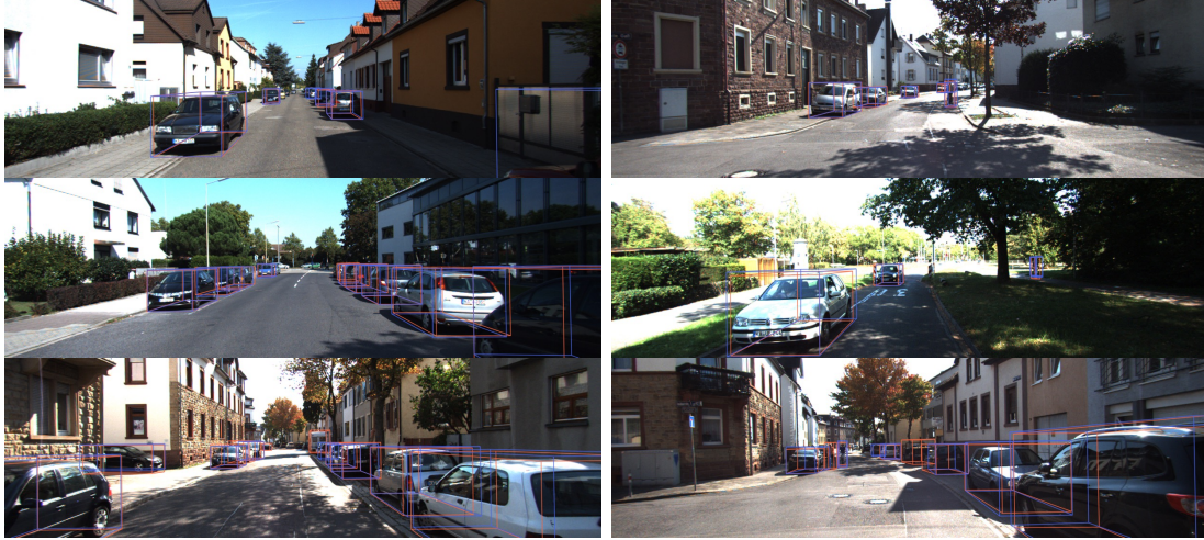
Figure 5. We visualize the results of 3D object detection using ImVoxelNet(+homo) on KITTI val set, where the orange represents the ground truth and our predicted results are colored in blue. The left column shows results of the network trained on the Car category only, and the right column is trained on three categories including Car, Pedestrian, and Cyclist. It is worth noting that, with the homography loss, it is possible to detect small targets and even truncated objects.
