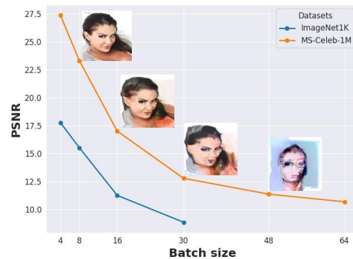
Figure 5. Effect of increasing batch size on the quality of image recovery. ImageNet and MS-Celeb-1M images are reconstructed in 224 \times 224 px and 112 \times 112 px respectively. Representative sample reconstructions are presented for batch sizes of 8, 16, 30 and 48. The maximum number of batch sizes is limited to 30 for ImageNet dataset amid GPU memory constraint.
