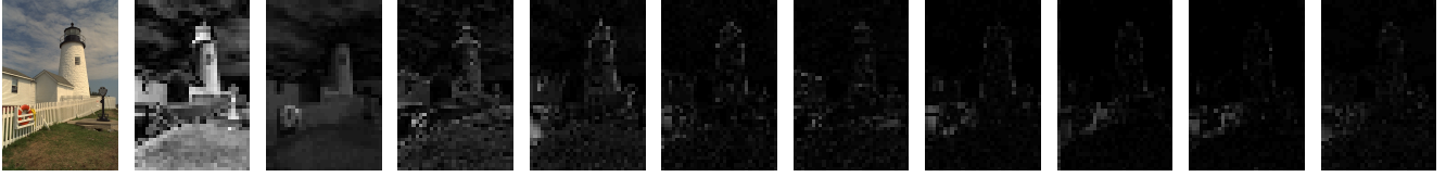
Figure 2. Visualization of sorted channels with the top-10 largest average energy. Left 1: the original image (kodim19.png). Lighter regions correspond to larger symbol magnitudes |\hat{y}| . It can be seen from the figures that most strong activation concentrates in the first channel (left 2) and the remained channels become sparse gradually.
