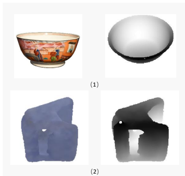
Figure 4. Complementary information in RGBD images for few-shot 6D pose estimation. (1) Texture information in RGB images is crucial cue for objects with smooth surface. (2) Geometric information in depth images is important cue for texture-less objects.
