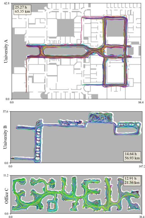
Figure 2. Inertial localization dataset contains IMU measurements and ground-truth locations based on Visual Inertial SLAM in three buildings. The ground-truth trajectories are shown here with random colors, overlaid on the respective floorplans. (Image dimensions are in meters).
