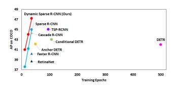
Figure 1. Performance vs. training epochs on the COCO 2017 validation set. All results are reported with single-scale inference using the ResNet-50 backbone. Our Dynamic Sparse R-CNN achieves the state-of-the-art 47.2% AP with the same 36 training epochs as Sparse R-CNN. Circles: Transformer-based methods. Triangles: CNN-based methods.
