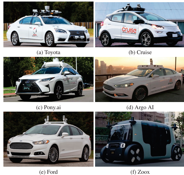
Figure 1. Different multi-LiDAR configurations used in different autonomous vehicles [1–6].
