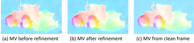
Figure 4. Example of MV comparison. We find MV is more accurate and more similar to the MV from clean frames after ME refinement. Zoom in for a better view.
