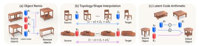
Figure 3. Our DT-Net framework learns a disentangled representation for the topology and shape, thus facilitating novel generation applications via disentangled manipulation on the topology code  $Z_T$  and/or the shape code  $Z_S$ , *e.g.*, (a) remix the shape and topology of two different objects; (b) object interpolation by manipulating the topology/shape code; and (c) arithmetic operations in the latent space.
