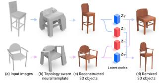
Figure 1. Our DT-Net learns to construct a *topology-aware neural template* (b) adapted to the input (a) and then deform it towards an accurate 3D mesh while preserving the initial (learned) topology. This decoupled design enables a disentangled latent representation of *topology* ( $\mathbf{Z}_T$ ) and *shape* ( $\mathbf{Z}_S$ ), promoting controllable 3D mesh generation, *e.g.*, remixing codes for object re-synthesis.
