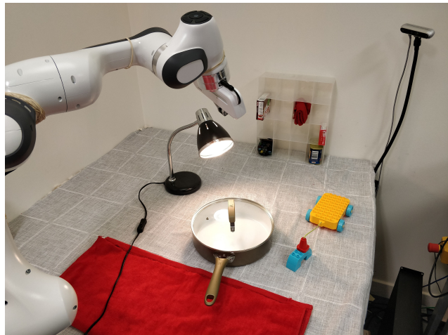
Figure 1. C2F-ARM learns sparsely-rewarded tasks with only 3 demonstrations. Real-world tasks include: turning on a light, pulling cloth from shelf, pulling a toy car, taking a lid off a saucepan, and folding a towel.
