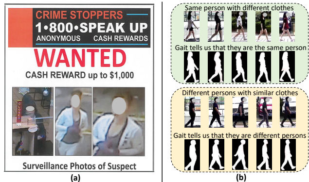
Figure 1. (a) shows a realistic wanted case that a suspect changed her coat from black to white for hiding. (b) reveals that the gait of person could help ReID, especially when the identity matching meets the cloth-changing challenge (All faces in the images are masked for anonymization).
