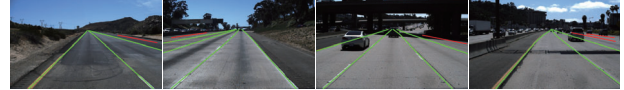
Figure 11. Detection results of the proposed algorithm on the TuSimple dataset. Detected lanes are depicted in green, while false negatives are in red.
