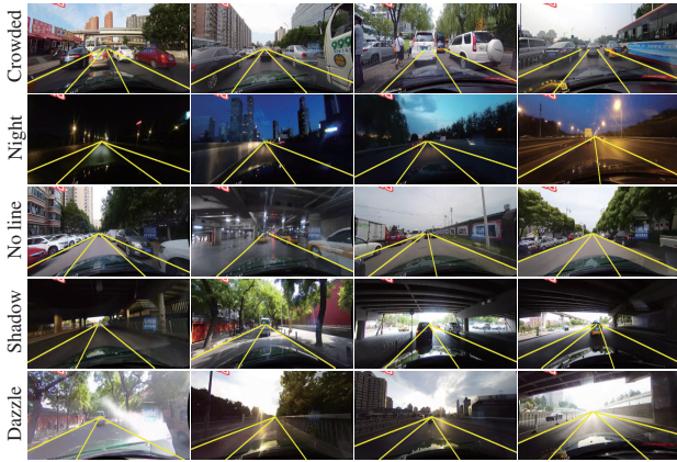
Figure 12. Detection results of the proposed algorithm on five challenging categories in the CULane dataset.
