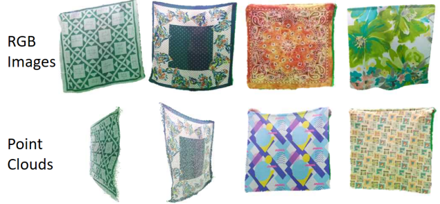
Figure 4. We record a new \phi -SfT real dataset of nine sequences with reference depth data to facilitate quantitative comparisons of monocular 3D surface reconstruction methods. Our setup consists of a synchronised RGB camera and an Azure Kinect. The depth camera provides depth maps serving as pseudo ground truth.
