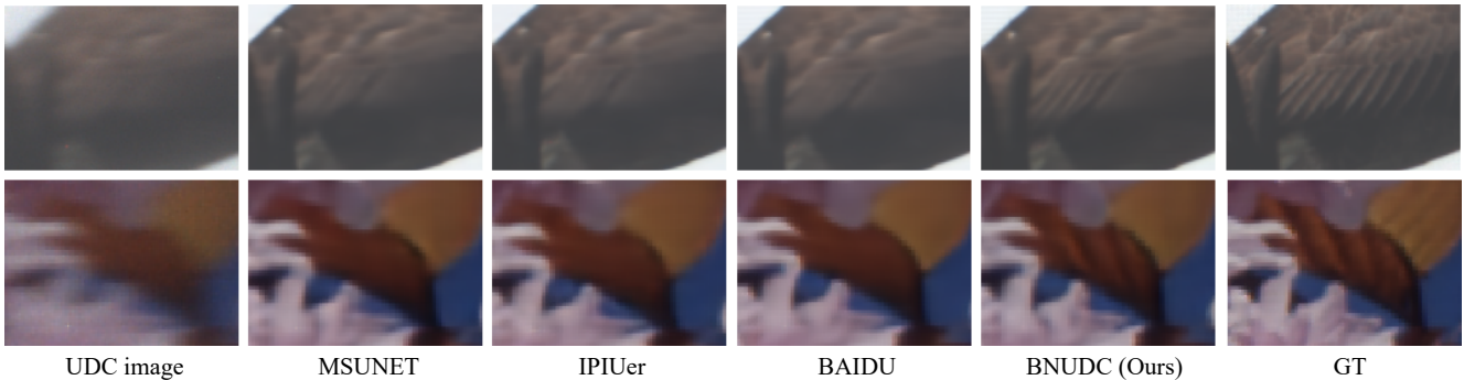
Figure 4. Two example images from the TOLED dataset restored by four networks. The first column contains the UDC images. Subsequent columns shows the reconstructed images obtained using MSUNET [40], IPIUer [39], BAIDU [39] and our BNUDC.
