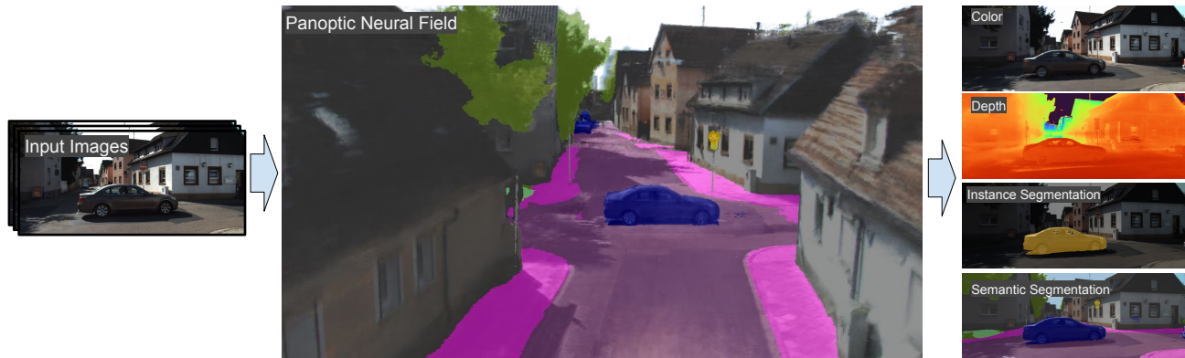
Figure 1. Panoptic Neural Fields (PNF) is an object-aware neural scene representation that decomposes a dynamic 3D scene into a set of objects ( things ) and background ( stuff ), each represented by a separate MLP based neural function. Our model predicts a panoptic-radiance field that represents the color, density, instance, and category label of any 3D point at any given time. The model is trained from RGB images alone and can describe dynamic challenging 3D scenes as shown above.
