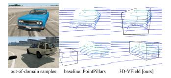
Figure 1. Predictions of PointPillars [18] trained on KITTI [13], without and with our adversarial augmentations on out-of-domain samples from the proposed CrashD dataset. CrashD comprises *rare* (top) and *damaged* (bottom) vehicles, resulting in natural adversarial examples [17]. As the models were applied to CrashD without fine-tuning, due to the different object shapes, the standard PointPillars delivered two false negatives and a false positive. *Images used with courtesy of BeamNG GmbH*.
