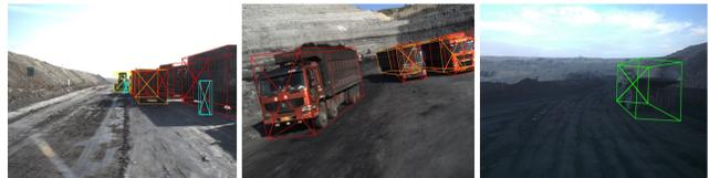
Figure 1. The environmental characteristics of the strip mine include rugged unstructured roads, the strong light exposure and dust. AutoMine annotates 3D objects with 9 degrees of freedom.
