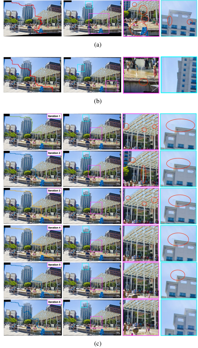
Figure 2. Stitched results using (a) the initial global alignment, (b) QR1A, (c) the iterative learning strategy of ACIS-QR1A.
