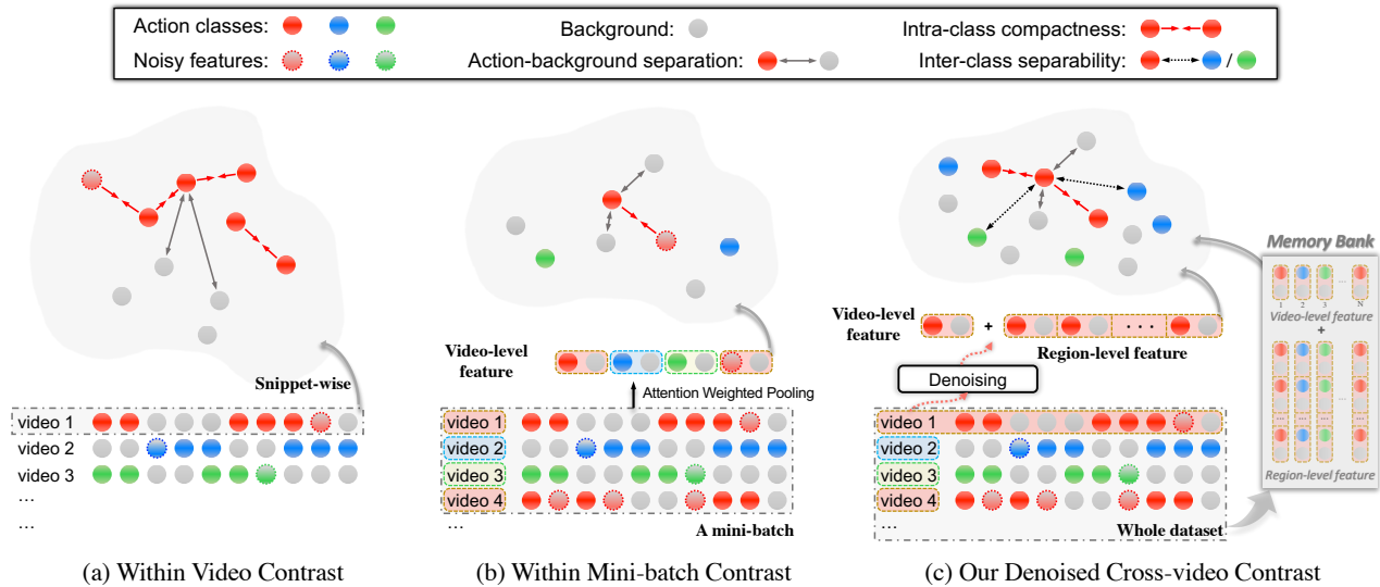
Figure 1. Different contrastive learning schemes. (a) Exploiting snippet-wise contrastive learning within single video to separate snippet-wise actions from backgrounds with pseudo-labels (e.g., [64]). (b) Exploiting deep metric learning within mini-batch to separate video-level actions from backgrounds with attention-weighted pooling (e.g., [36,41]). (c) Our denoised cross-video contrastive algorithm with 1) pseudo-label denoising module, 2) region-level feature contrastive learning across entire dataset, and 3) action-background separation, as well as intra-class compactness & inter-class separability.
