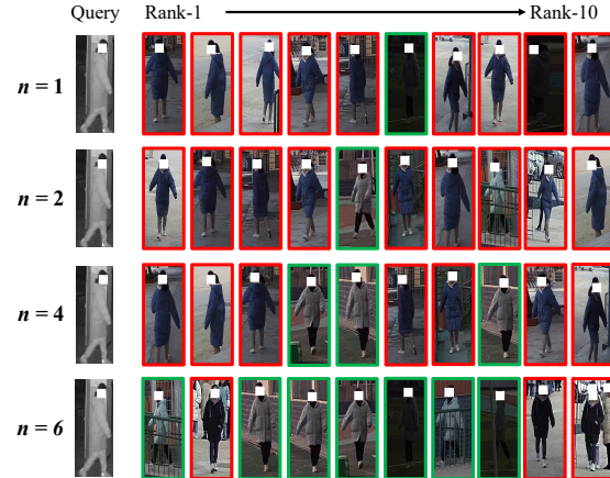
Figure 7. The visualization results on different settings, where n denotes the number of images in one tracklets. Obviously, image-based methods ( n = 1 ) cannot report satisfying results when two identities enjoy similar appearances, while video-based methods show noticeable performance with the enhancement of temporal information.
