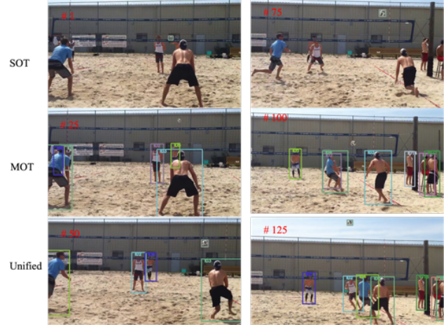
Figure 4. Visualization of our results on the challenging sequences in different tracking modes. Best viewed with zooming in. In the unified tracking mode, the specified volleyball is tracked together with multiple persons.
