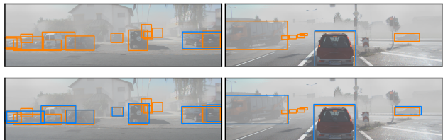
(b) Detections in foggy weather without (top) and with (bottom) DUA. We overlay the detection results (blue) and the ground truth (orange).
