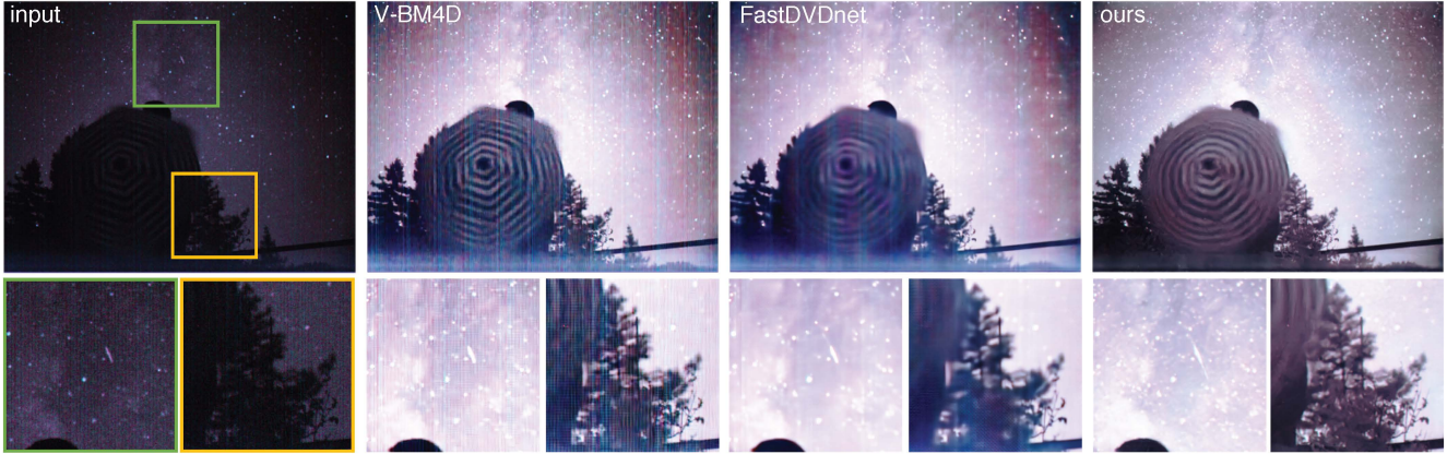
Figure 6. Results on noisy video clips taken at 10 fps in 0.0006 lx. The input sequence (left), V-BM4D, pretrained FastDVDnet, and our results are shown. Our method maintains more details throughout the clip and does not contain the prevalent streaking artifacts that are present in V-BM4D and the pretrained FastDVDnet. See supplement for full video clips. (Digital zoom recommended.)
