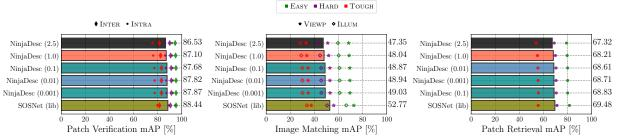
Figure 5. HPatches evaluation results. We compare the baseline SOSNet [74] vs. NinjaDesc, with 5 different levels of privacy parameter  $\lambda$  (indicated by the number in parenthesis). All results are from models trained on the *liberty* subset of the UBC patches [22] dataset.
