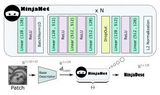
Figure 2. Top: Architecture of our content-concealing *NinjaNet* encoder  $\Theta$ . Bottom: A base descriptor with dimensionality *C* is transformed to *NinjaDesc* of the same size, *e.g.* C = 128.
