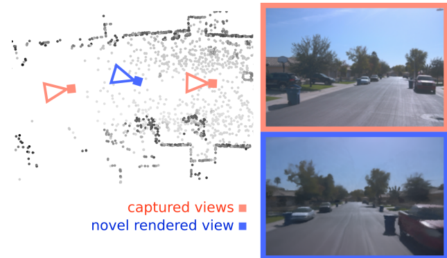
Figure 1: Neural Point Light Fields encode the information of a Light Field representation of a scene on a point cloud capture. An image is rendered for each camera ray based on the local encoding of the Light Field on relevant points.
