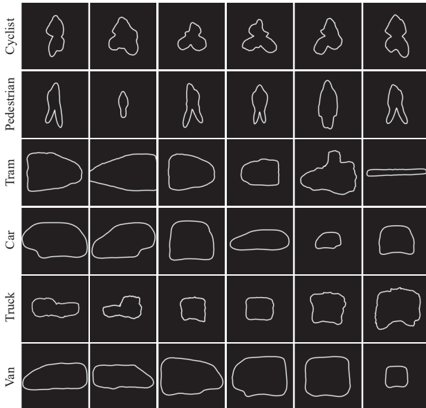
Figure 7. Visualization of contour centroids in the 16-dimensional eigencontour space, according to object categories. Although the centroids are determined by grouping training data in the lower-dimensional space, each centroid represents the structure of the corresponding object category faithfully.
