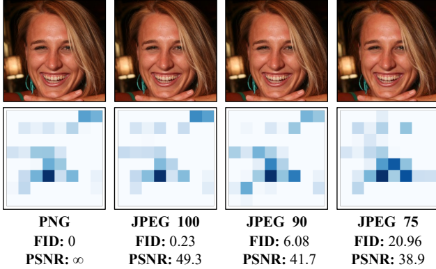
Figure 6. Effects of JPEG compression on an image. We show a sample FFHQ [33] image, saved with lossless PNG and different JPEG compression ratios. The FID scores under the images are calculated between FFHQ images saved using the corresponding JPEG format and the PNG format. PSNR is computed with 1000 images. While the images are perceptually similar, this induces changes in the Inception-V3 activations, resulting in large FID.
