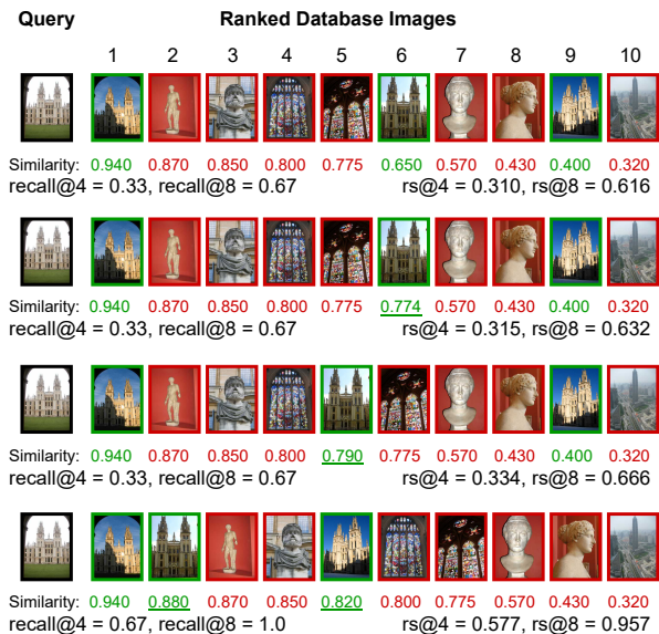
Figure 1. A comparison between recall@k and rs@k, the proposed differentiable recall@k surrogate. Examples show a query, the ranked database images sorted according to the similarity and the corresponding values for recall@k and rs@k and their dependence on similarity score change. Note that the values of recall@k and rs@k are close. Changes to similarity and ranking in some cases may not affect the original recall@k but can affect the surrogate, with the latter having a more significant impact than the former. Similarity values of all negatives are fixed for ease of understanding. The similarity values of the positives that were changed in rows 2, 3 and 4 are underlined .
