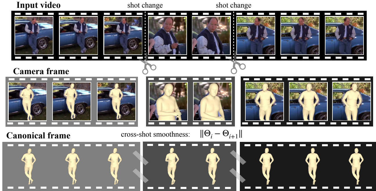
Figure 1. Human Mesh Recovery from Multiple Shots. Videos from edited media, like movies, include sudden shot changes that lead to discontinuities between the frames (top), which reduce the rich potential of a film to a series of short independent temporal sequences. However, within the same scene, the underlying 4D structure of the scene changes smoothly. We leverage this insight and treat the different shots as multi-view cues that provide complementary information about the 3D human body underlying these shot boundaries. This leads to both more accurate 3D reconstructions (middle, bottom) and longer 3D pose sequences. These serve as a great source of data for training deep learning models that enable direct human mesh recovery on movie data.
