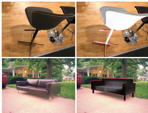
Figure 1. Given a single input photograph (left) and a known 3D model, our approach accurately estimates the 6D camera-object pose together with the focal length of the camera (right), here shown by overlaying the aligned 3D model over the input image. Our approach handles a large range of focal lengths and the resulting perspective effects.
