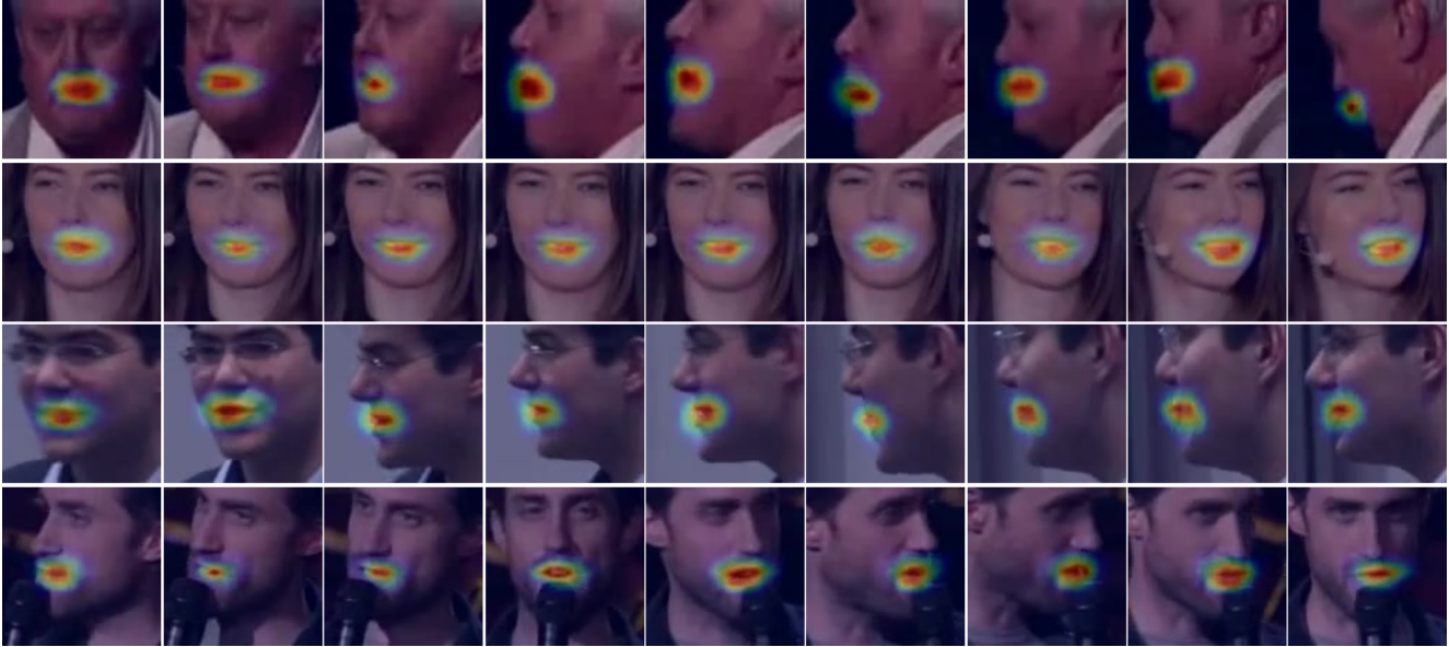
Figure 2. Visualization of the visual attention masks \alpha from the VTP module superimposed on the input frames that produce them. The video clips used here are random samples from the LRS3 dataset. It is evident that the model follows the more discriminative mouth region.
